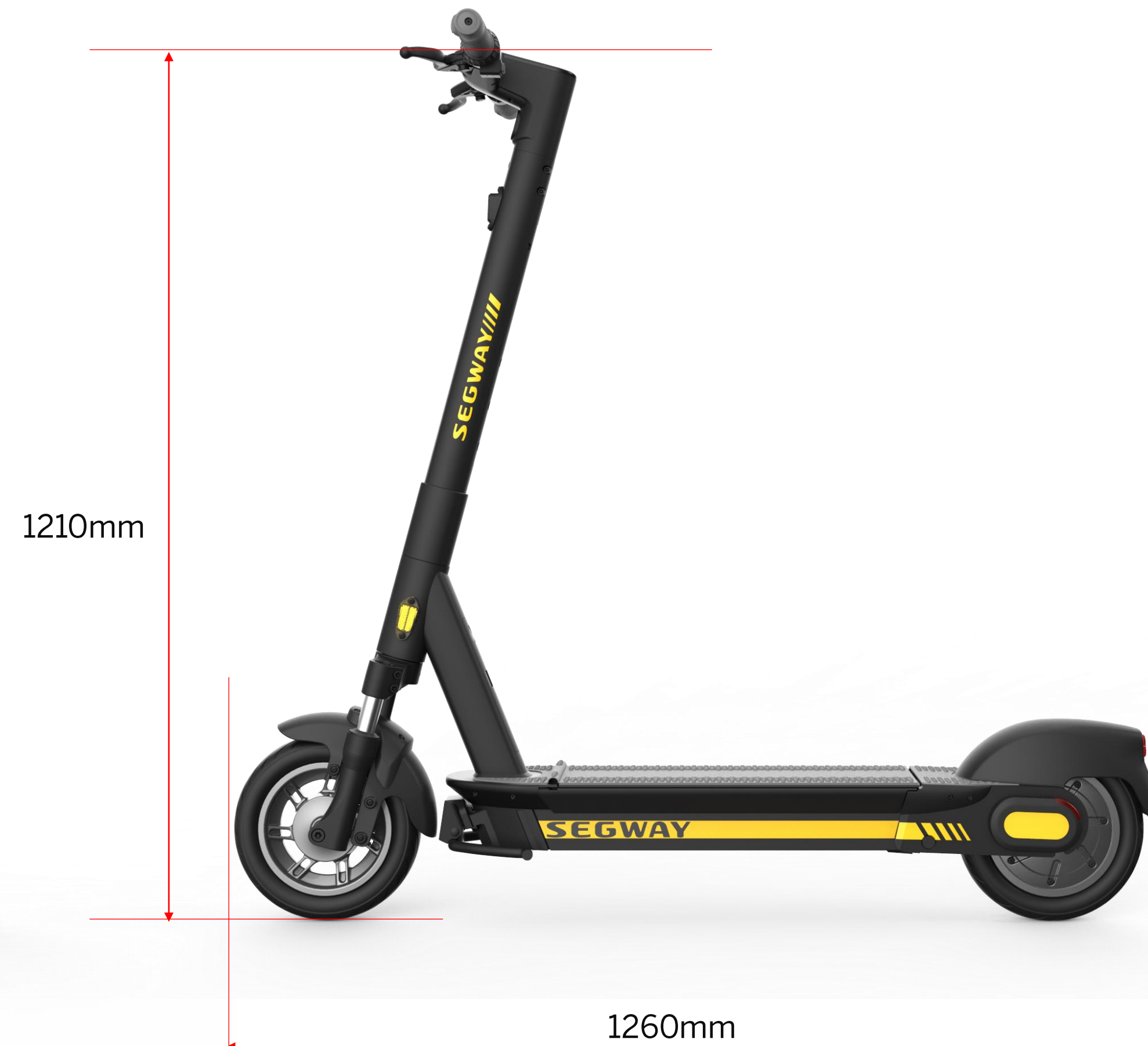
Rear suspension version ( 10 inch front tire/ 10 inch rear tire ) 1260mm×555mm×1210mm
