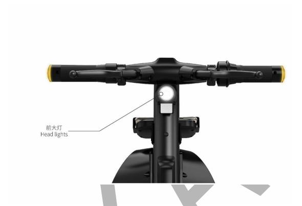
OKAI scooter is equipped with a headlamp at the front of the scooter, which will light up automatically when the scooter is unlocked.
