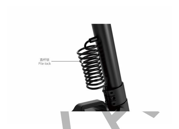
There is a stem lock at the lower end of the front pipe, which is used to lock the scooter on the parking post. The IOT of the sample scooter is in the test mode. When you press and hold the button for more than 1 s to unlock the scooter, the stem lock will automatically be unlocked. In formal order, customers need to unlock the stem lock through commands.
