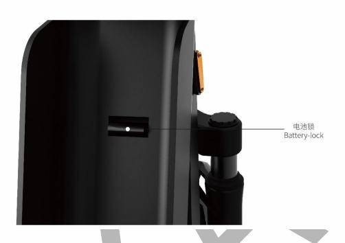
The battery lock of OKAI scooter can be directly controlled by the IOT. Through CAN bus, the IOT sends the unlocking command to the battery lock. When the battery lock is opened, the battery will pop up automatically. As long as you press down the battery cover, it will automatically lock.
